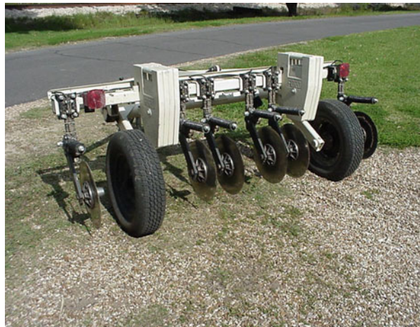
Figure 1. Veris® 3100 Soil EC Mapping System.
