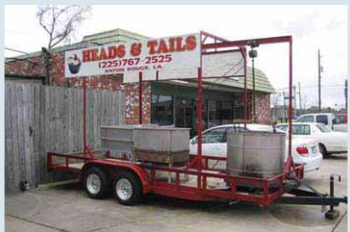
Figure 10.8. Custom mobile crawfish boiling rig used for catering large crawfish boils.
