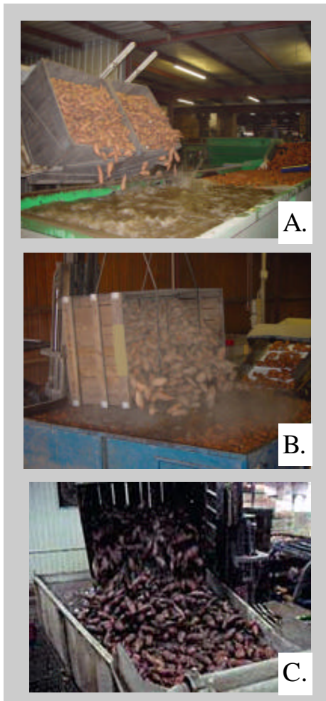
Fig 4. An example of roots being dumped properly into water (A) and examples of roots being dumped into a dump tanks that were overfilled with sweetpotatoes resulting in large impacts of one sweetpotato onto another (B and C).
